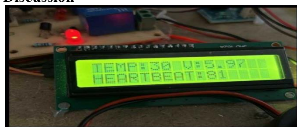
Fig 5.2: Temperature, Heartbeat, and Solar Voltage Displayed on LCD
