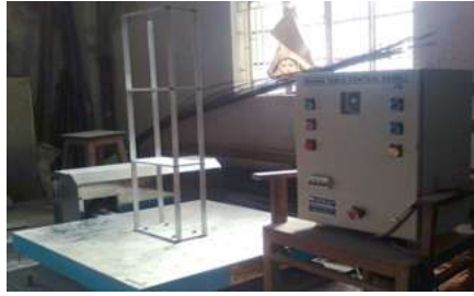
Fig. 15. Experimental set up for the Shake table test.
