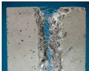
Steel fiber reinforced concrete
