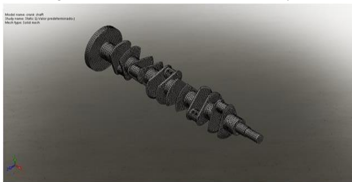
Fig 2. 3D Finite Element Representation in SOLIDWORKS
