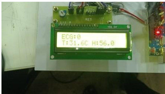
Figure 5: Fig6- LCD-Based Real-Time Display of ECG, Temperature, and Humidity Parameters in an Embedded Health Monitoring System
