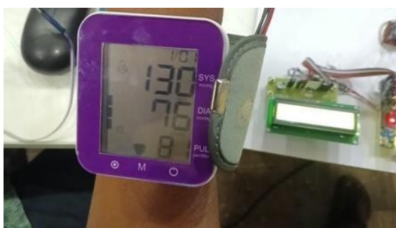
Figure 5: Fig.7-Wrist-Worn Digital Blood Pressure Measurement Integrated with an Embedded Health Monitoring Setup
