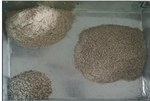
Figure 4.2: Sieved Steel Slag Samples Classified by Particle Size
