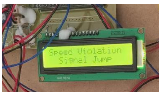
Figure 4. LCD Display Showing Signal Jump and Speed Violation Alert.
