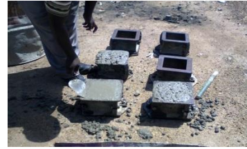
Filling the mould (for 150 mm cube 3 equal layers)
