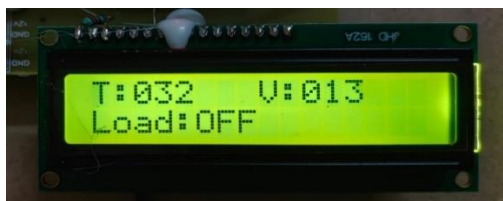
Figure 6. LCD Display Showing Solar Panel Monitoring Parameters.
